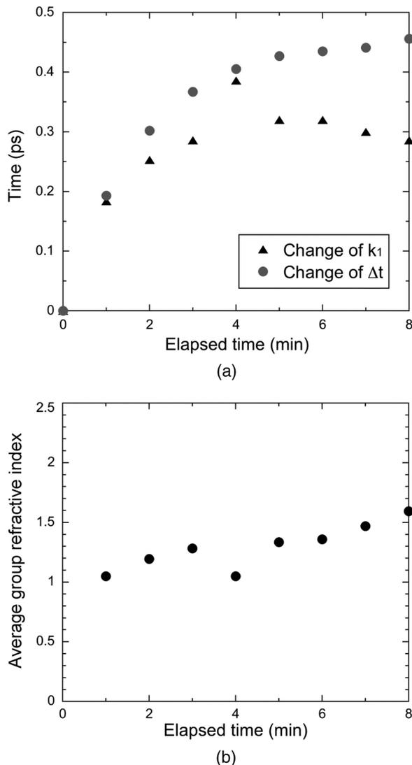
Fig. 9. Temporal change of each parameter for wet paint film with respect to elapsed time. (a) Deviations of  $\Delta t$  and  $k_1$  from the initial values at 0 min and (b) average group refractive index.
