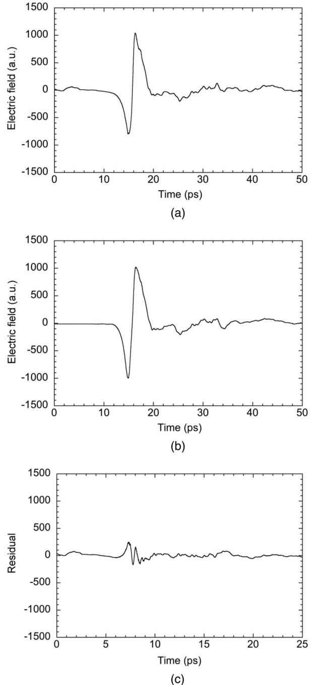
Fig. 4. Temporal waveform of the THz echo pulse of a single-layer dry paint film with 60  $\mu\text{m}$  thickness. (a) Signal measured with THz paint meter, (b) signal simulated by multiple-regression analysis, and (c) residual between the measured signal and simulated signal.
