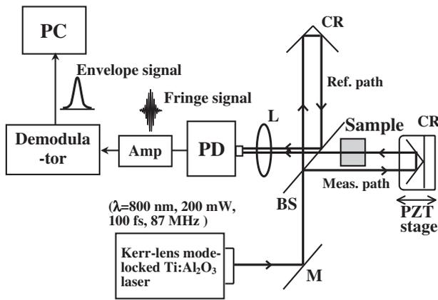
Fig. 2. Experimental setup of femtosecond pulse interferometry. M: mirror, BS: beam splitter, CR: corner reflector, PZT stage: piezoelectric stage, L: lens, PD: photodetector, Amp: amplifier, PC: personal computer.
